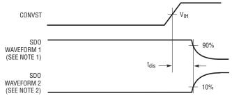
NOTE 1: WAVEFORM 1 IS FOR AN OUTPUT WITH INTERNAL CONDITIONS SUCH THAT THE OUTPUT IS HIGH UNLESS DISABLED BY THE OUTPUT CONTROL NOTE 2: WAVEFORM 2 IS FOR AN OUTPUT WITH INTERNAL CONDITIONS SUCH THAT THE OUTPUT IS LOW UNLESS DISABLED BY THE OUTPUT CONTROL
